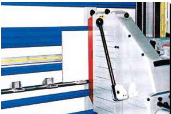
Supporto intermedio ribaltabile Intermediate turnover support
